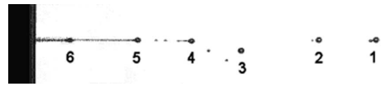
FIG. 7. Distorted droplet formation. Droplets 1 and 2 are standard droplets, droplet 3 corresponds to a disturbance of the acoustical signal (such as, e.g., seen in Fig. 6 for droplets number 34–36 of that figure). Here droplets 4–6 are standard again, but an air bubble is now present in the nozzle. After hundreds of cycles, this can lead to the breakdown of the jetting process.
